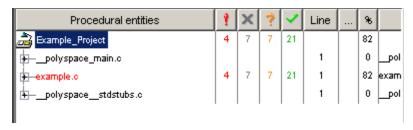
The file example.c is red because its has a run-time error. PolySpace software assigns a file the color of the most severe error found in that file. The first column of the table is the procedural entity (the file or function). The following table describes some of the other columns in the procedural entities view.
